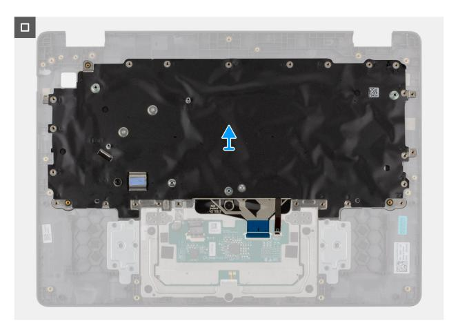
Figure 51. Removing the keyboard
