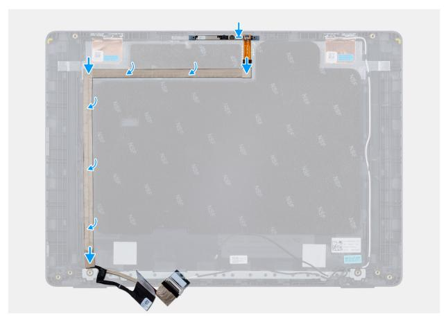
Figure 85. Installing the eDP cable
