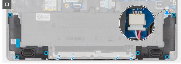
Figure 28. Installing the speakers
