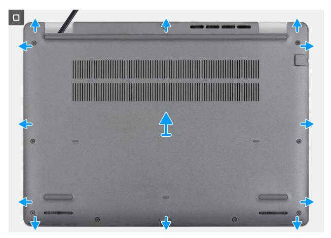
Figure 12. Removing the base cover
