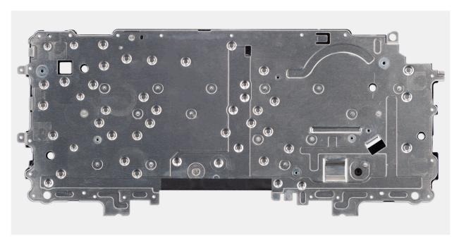
Figure 57. Removing the keyboard support plate
