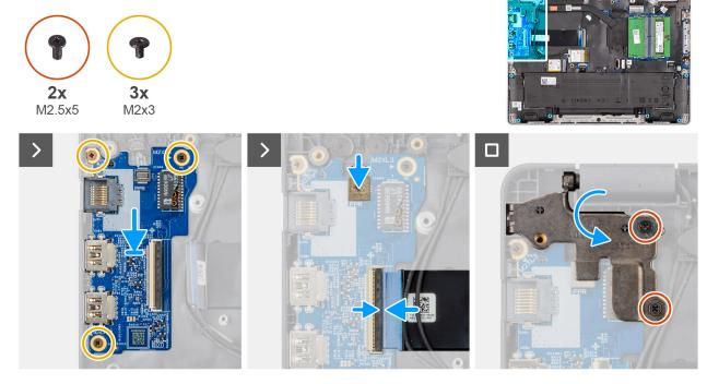
Figure 37. Installing the I/O board
