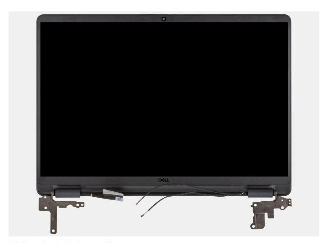
Figure 64. Removing the display assembly
