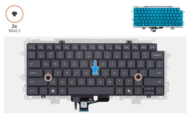
Figure 59. Installing the keyboard support plate
