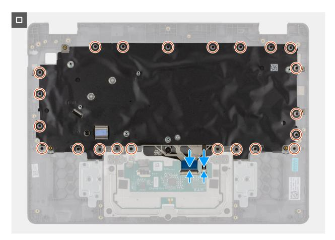
Figure 55. Installing the keyboard
