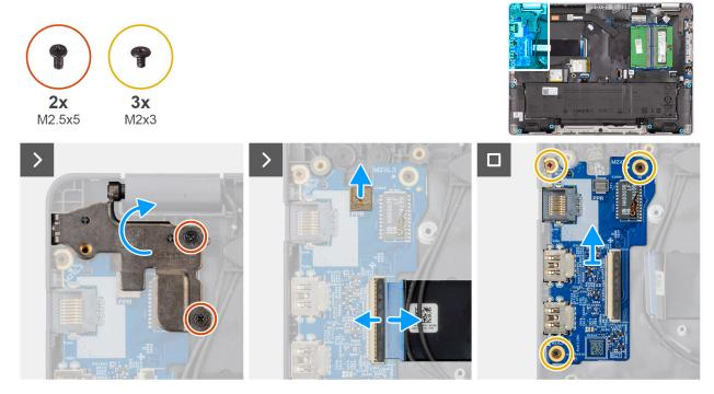
Figure 36. Removing the I/O board
