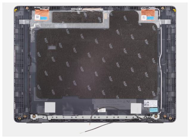
Figure 87. Installing the display back-cover assembly
