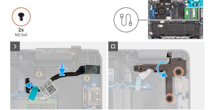
Figure 33. Installing the power-adapter port
