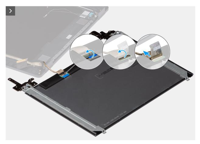
Figure 76. Removing the display-panel assembly
