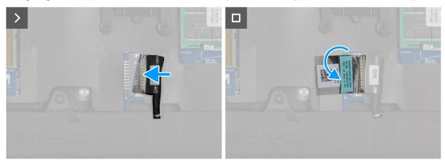
Figure 14. Connecting the battery cable
