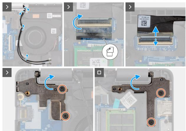
Figure 62. Removing the display assembly
