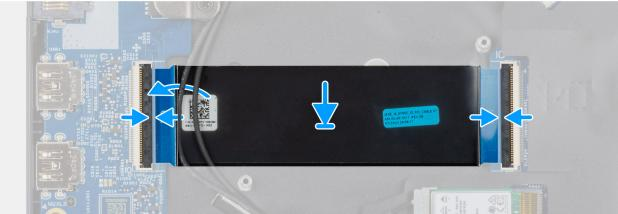
Figure 39. Installing the I/O board
