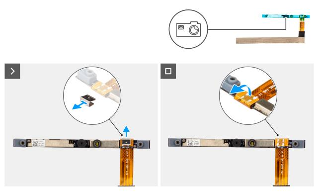
Figure 82. Removing the camera
