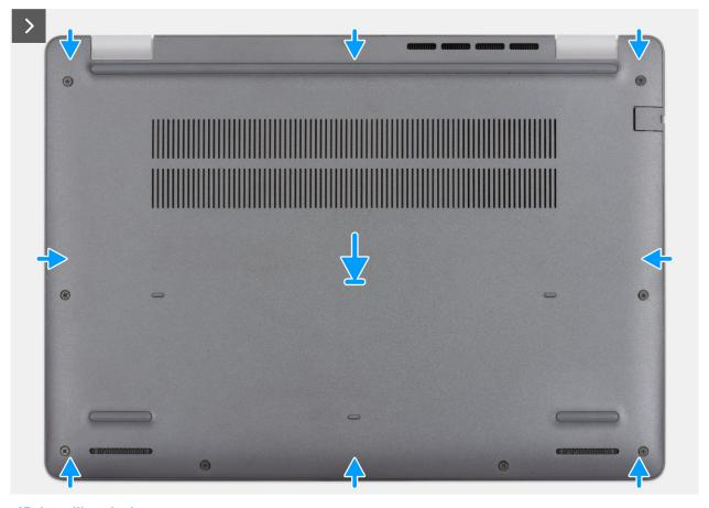
Figure 15. Installing the base cover
