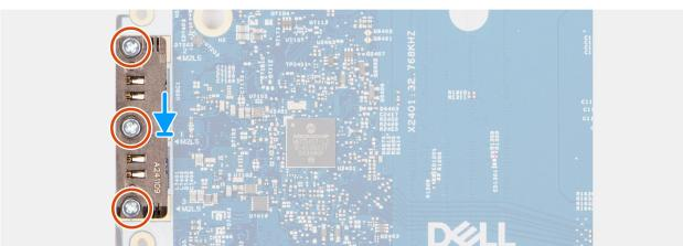
Figure 49. Installing the USB Type-C module
