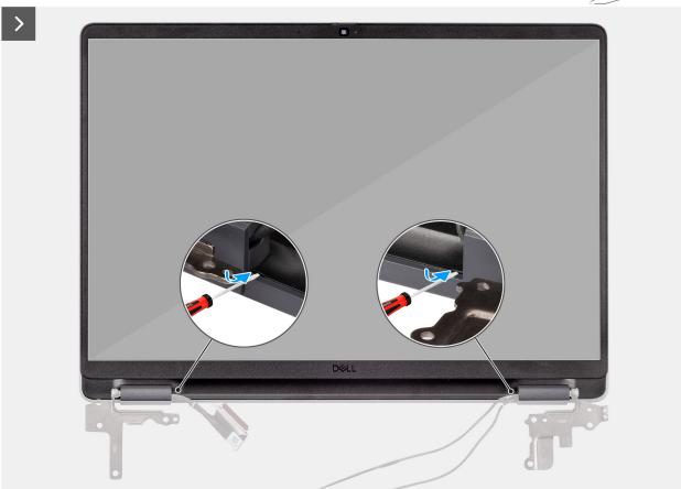
Figure 67. Removing the display bezel
