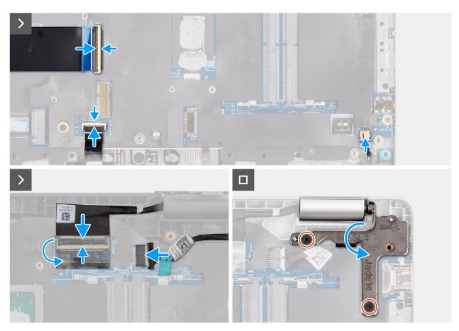
Figure 47. Installing the system board
