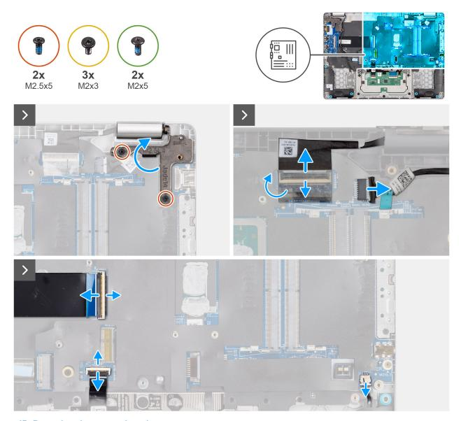
Figure 43. Removing the system board
