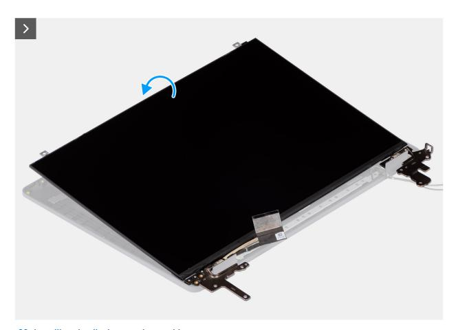
Figure 80. Installing the display-panel assembly
