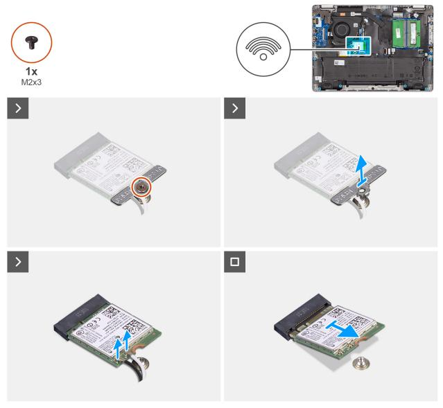
Figure 25. Removing the wireless card
