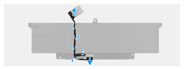
Figure 19. Removing the battery cable
