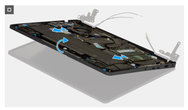
Figure 63. Removing the display assembly
