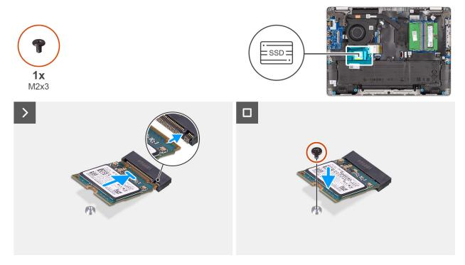
Figure 24. Installing the SSD
