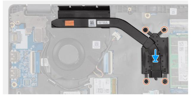
Figure 35. Installing the heat sink
