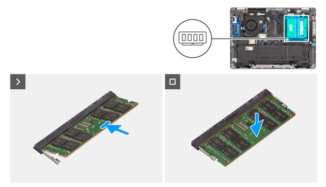
Figure 22. Installing the memory module
