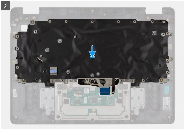
Figure 54. Installing the keyboard
