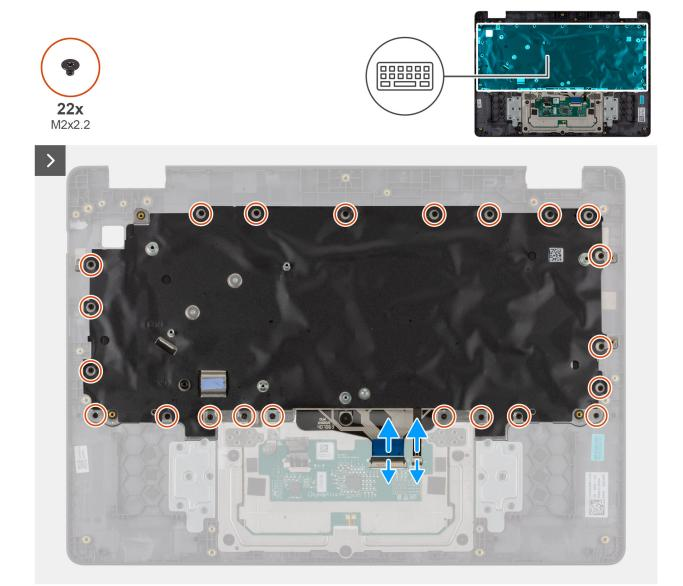
Figure 50. Removing the keyboard
