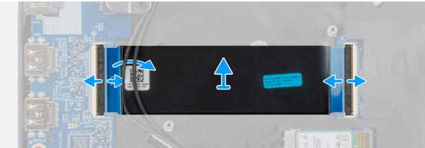
Figure 38. Removing the I/O-board FPC cable
