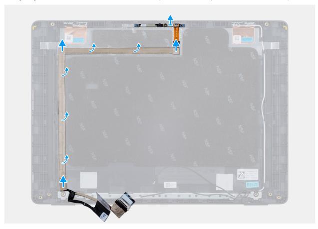
Figure 84. Removing the eDP cable
