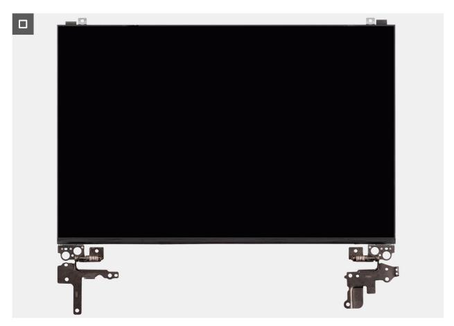
Figure 77. Removing the display-panel assembly
