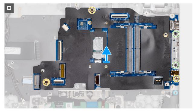
Figure 44. Removing the system board
