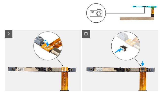
Figure 83. Installing the camera
