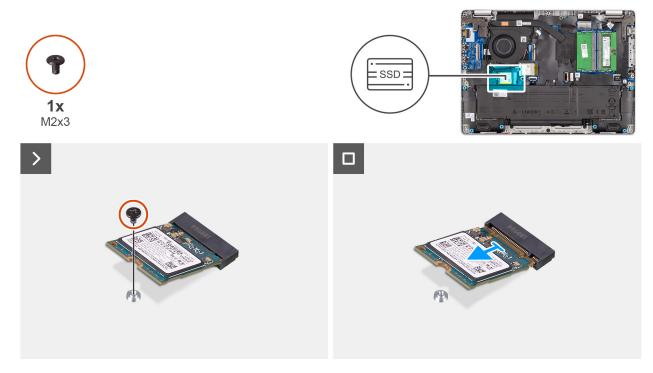
Figure 23. Removing the SSD
