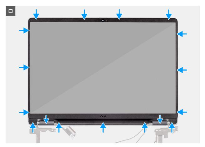
Figure 73. Installing the display bezel
