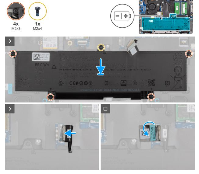
Figure 18. Installing the battery
