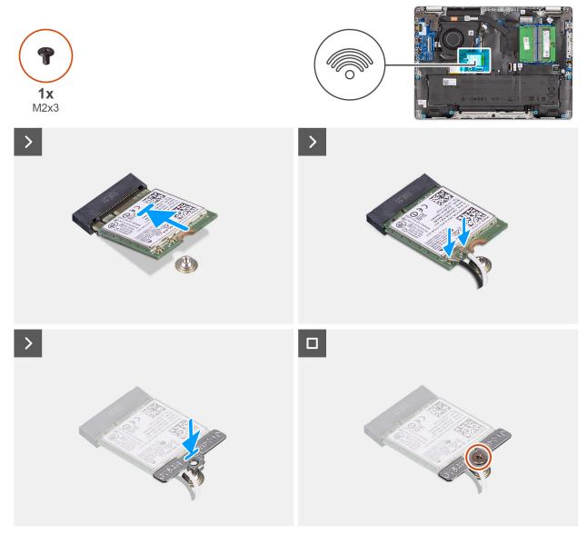
Figure 26. Installing the wireless card
