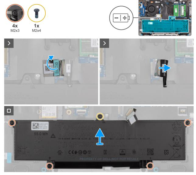
Figure 17. Removing the battery
