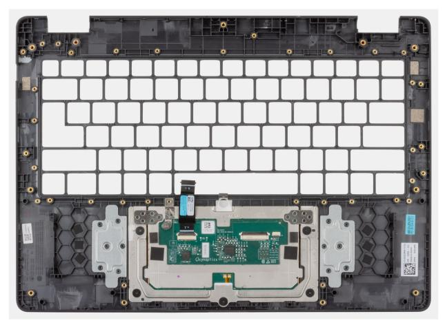
Figure 61. Installing the palm-rest assembly
