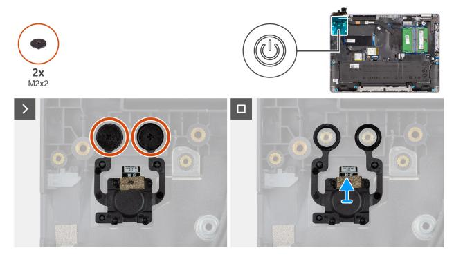
Figure 40. Removing the power button with fingerprint reader
