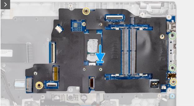
Figure 46. Installing the system board
