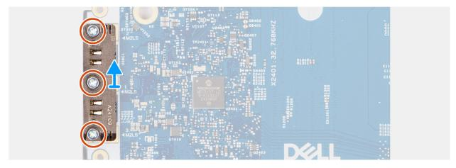
Figure 48. Removing the USB Type-C module
