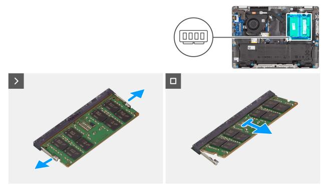
Figure 21. Removing the memory module
