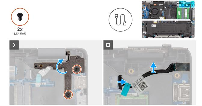
Figure 32. Removing the power-adapter port
