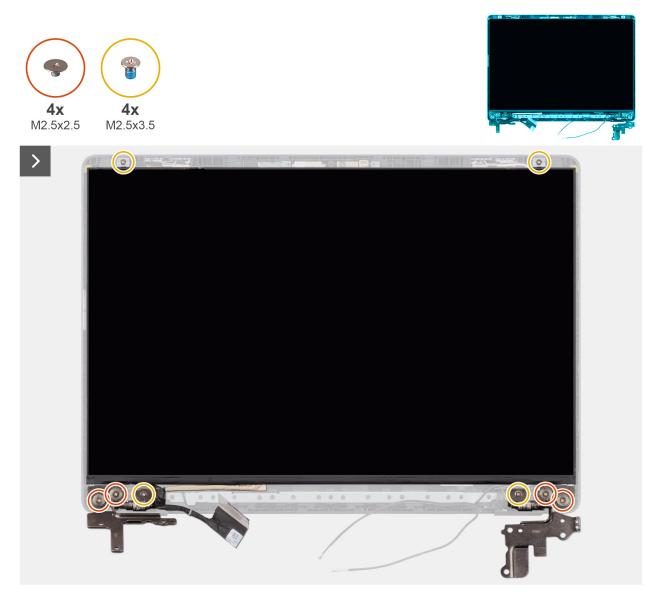
Figure 74. Removing the display-panel assembly
