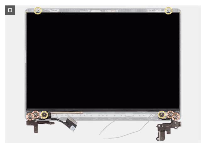
Figure 81. Installing the display-panel assembly
