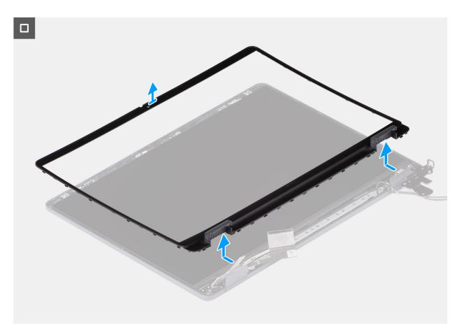
Figure 71. Removing the display bezel
