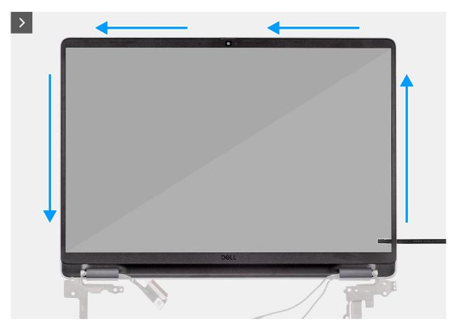
Figure 70. Removing the display bezel
