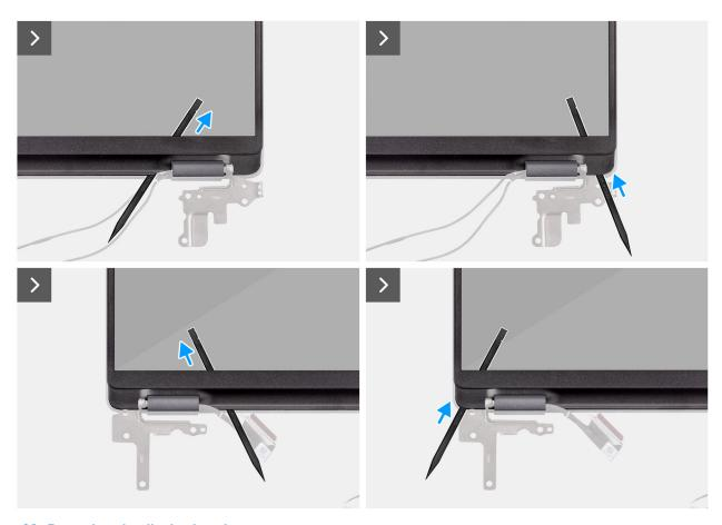
Figure 69. Removing the display bezel
