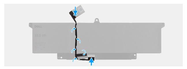
Figure 20. Installing the battery cable
