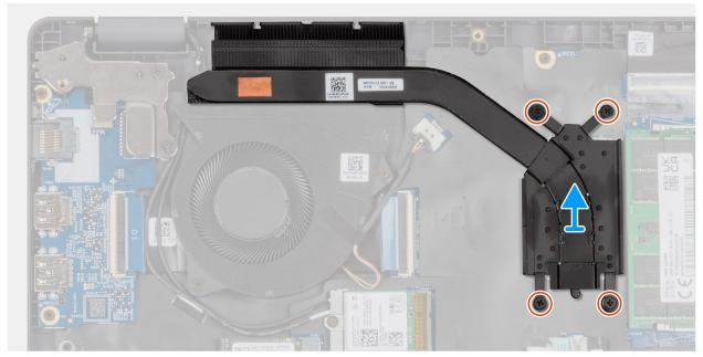
Figure 34. Removing the heat sink
