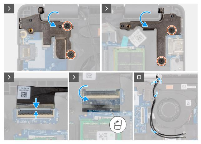
Figure 66. Installing the display assembly
