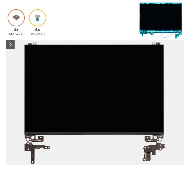
Figure 78. Installing the display-panel assembly
