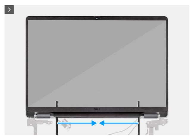
Figure 68. Removing the display bezel
