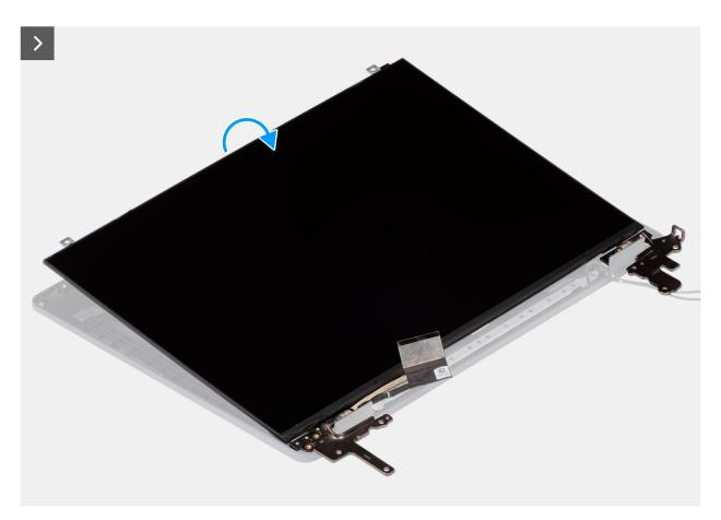
Figure 75. Removing the display-panel assembly
