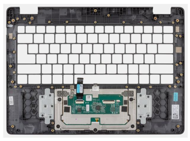
Figure 60. Removing the palm-rest and assembly
