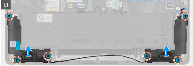
Figure 27. Removing the speakers
