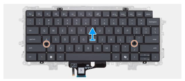
Figure 56. Removing the keyboard support plate
