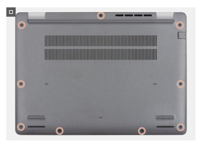
Figure 16. Installing the base cover
