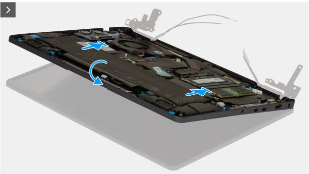
Figure 65. Installing the display assembly
