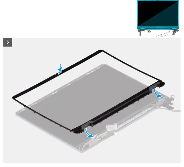
Figure 72. Installing the display bezel
